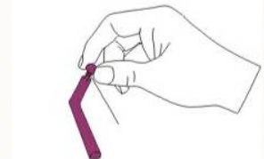
6 - Remove the knobs on the top to insert the new string in the small hole on the knob.
